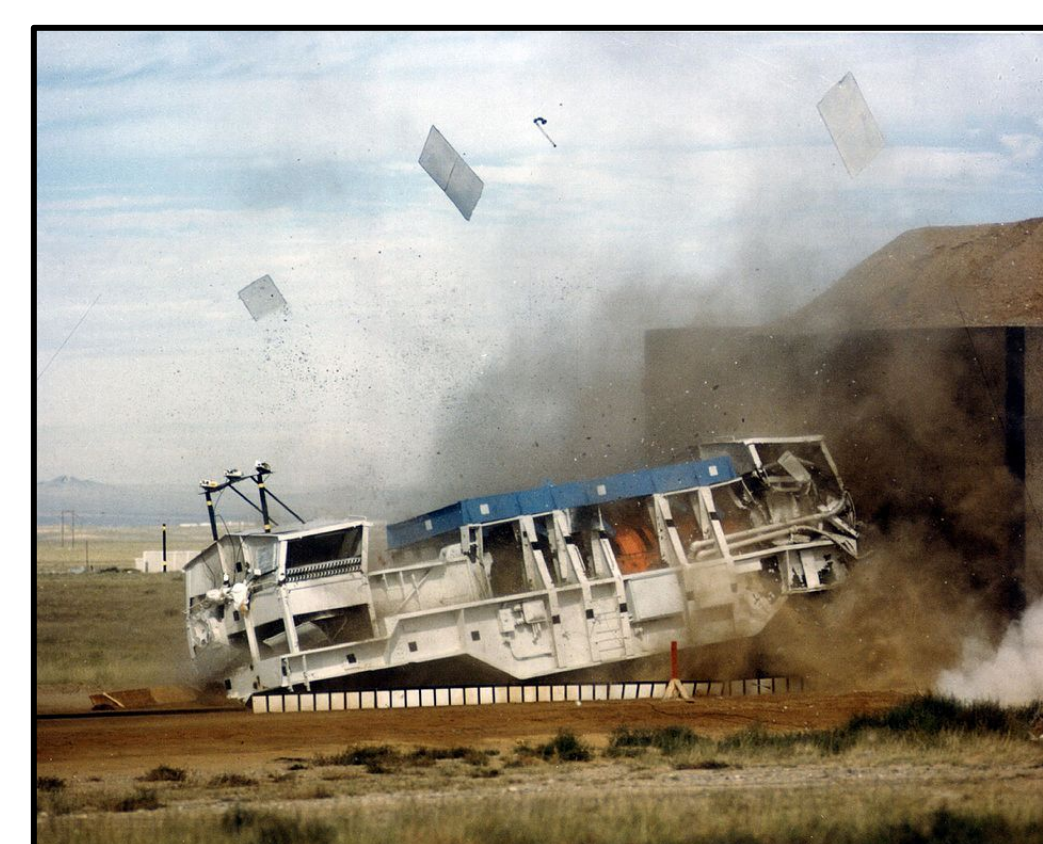
Fig.1. Spent Nuclear Fuel cask testing by Sandia Laboratories (cask was propelled into wall at 81 mph and remained intact)
