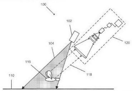
Abstract: A method for detecting an airborne object. Electromagnetic radiation is emitted from a transmitter to overlap with a receiver's field of view. When an airborne object enters the field of view, the electromagnetic radiation interacts with moving airfoils on the airborne object to produce reflected and scattered electromagnetic radiation. The reflected and scattered electromagnetic radiation is analyzed to detect, classify and/or determine the orientation of the airborne object.
