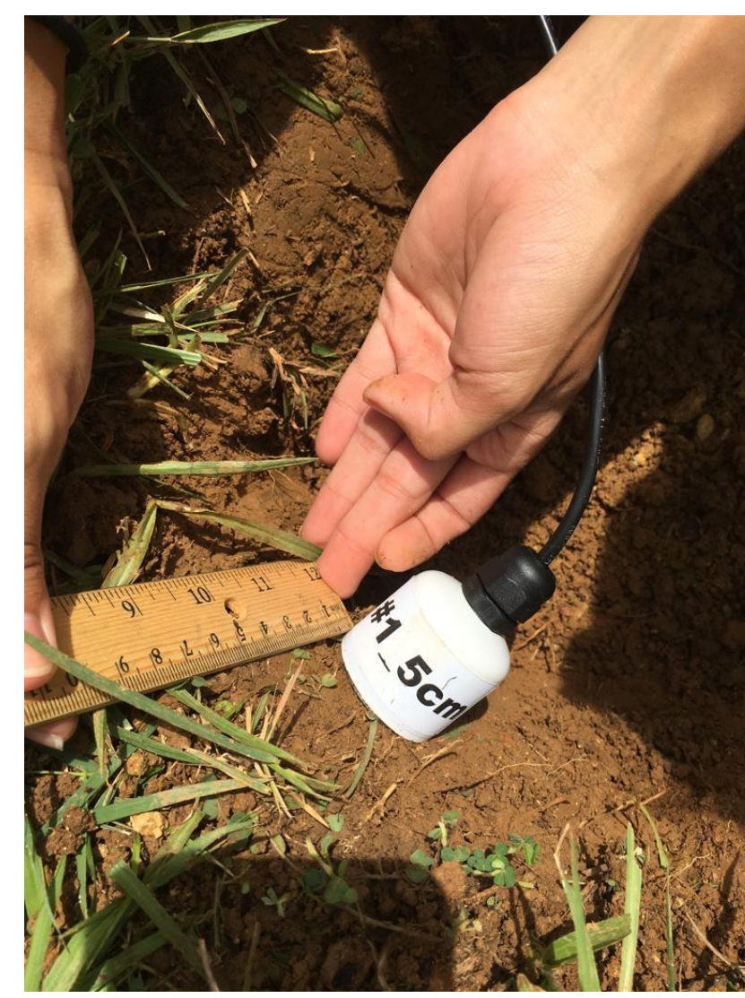
Figure 1: Hydra Probe Soil Sensor at 5 cm below the ground.
