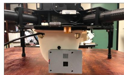
Figure 4: 3D printed mount installed as the DJI M100's Payload
