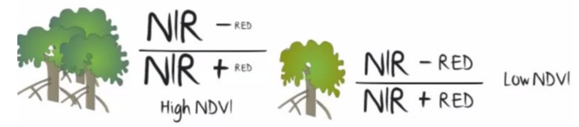
Figure 4. A schematic illustration of NDVI
