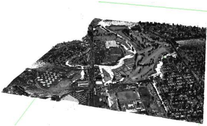
Figure: 3D LiDAR point cloud graphed by intensity for a location close to the JFK airport, NY.
