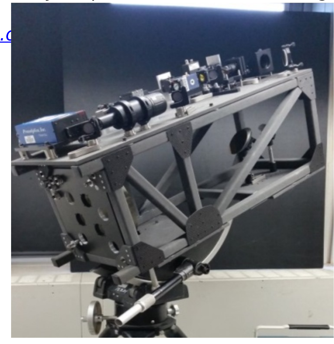
Figure 3: This is an image of the CCNY Ground Based Infrared LIDAR that was used to collect the data. Courtesy of Morann Dagan.
