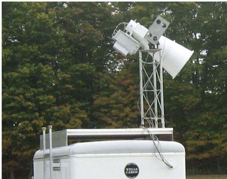
Figure 5: NOAA-CREST L-Band radiometer for soil moisture measurements ( http://crest.cuny.cuny.edu/facilities )
